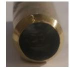
**Step 4: Cleaning up the Taper on the Case** Again, placing in the horizontal drill and using a metal file, I just cleaned up the taper, removing the burs from where it had been cut off.
