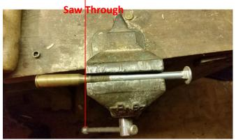
Step 2: Cutting off the percussion cap It is tempting to cut off the cap at the point where the groove in the casing is, I learnt to my cost that this is not far enough in to take off the whole cap.
