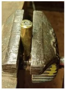
Step 2: Cutting off the percussion cap (cont) In reality you need to cut off the cap about 6mm from the end. See picture bottom right for amount to take off.
